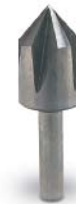
Countersink bit —drills a neat taper for the head of a wood screw
