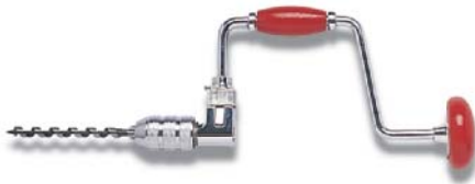
Brace —bores holes in wood by hand. Special auger bits must be used with the brace.
