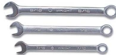
Combination wrench —has both box and open-end heads. Both ends are for the same size bolt.
