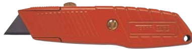
Utility knife —for safety, the blade can be retracted into the handle.
